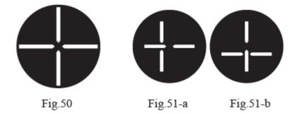
c. When the vertical lines are seen disposed as shown in Fig.51-a, turn rotation prism (2) of the left eye with 0 scale upward. Then turn prism rotation knob (1) slowly so that the image is shown as Fig.50 (horizontal phoria).
