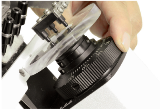
Fig 7.5 Astigmatism axis measuring hand wheel
