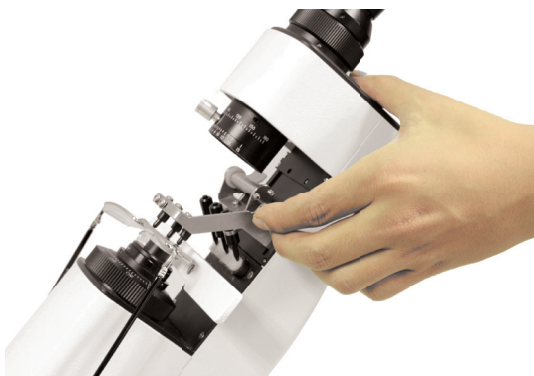
Fig 7.3 Lens pressing unit
