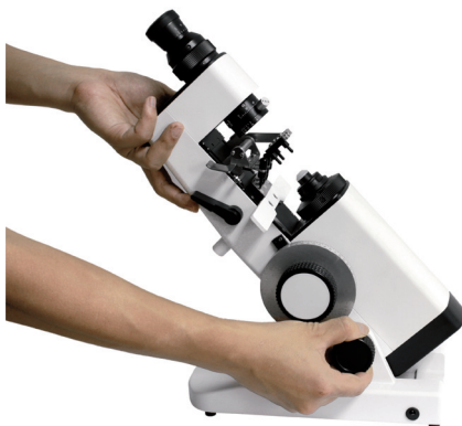
Fig7. 8 Instrument's inclination Lever
