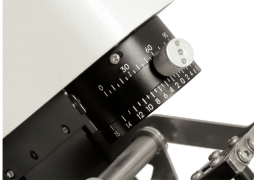
Fig 7.2 Prism compensation device
