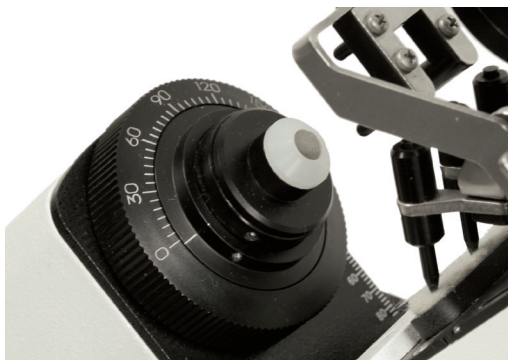
Fig 7.4 Objective lens bearing seat
