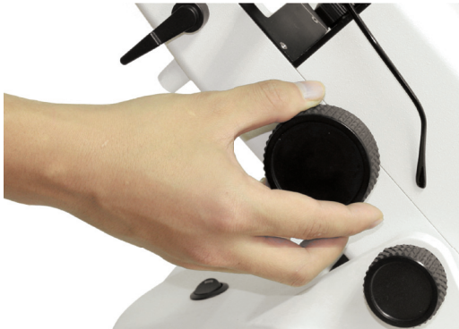
Fig7. 12 Diopter measuring handwheel
