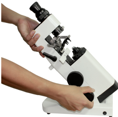
Fig7. 8 Instrument's inclination Lever
