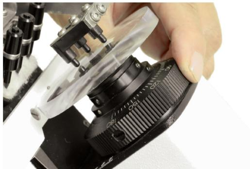
图 7.5 散光轴位测量手轮
